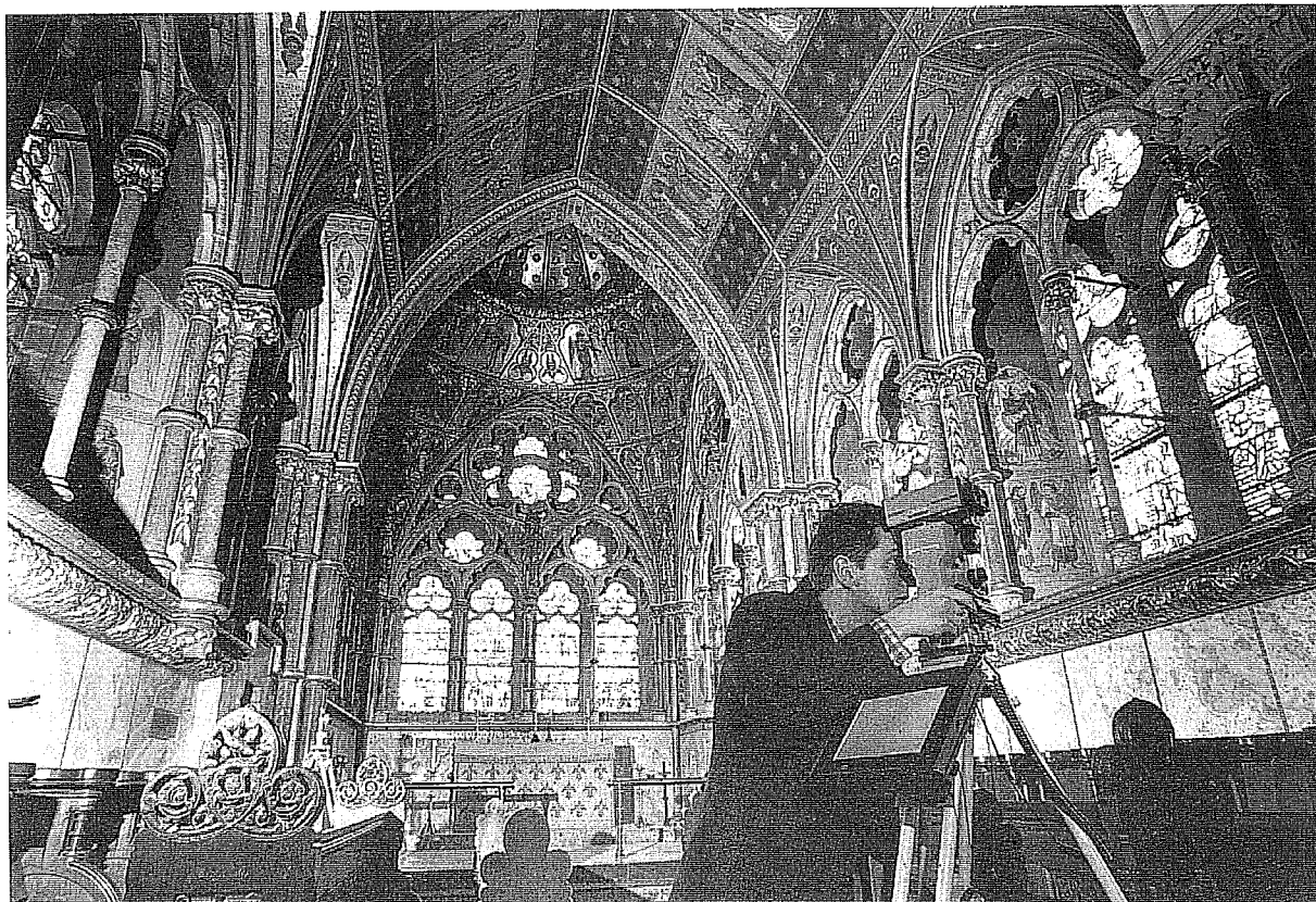
Plate 10. T1000 electronic theodolite with Leica 3002S REDM with realtime data logging to PenMap (Reproduced by kind permission of the Guardian. Photograph: Don McPhee)
